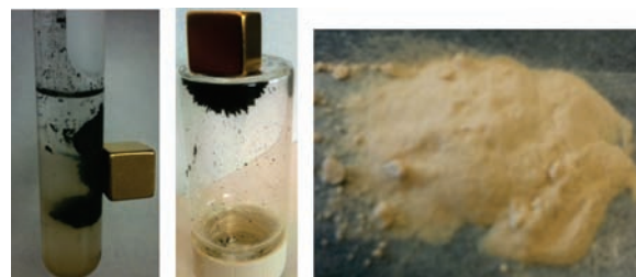
Figure 2. (a) Sequestration utilizing catalyst-activated Nb-tagged Co/C; (b) spent magnetic oligomer; and (c) Nb-tagged Si particles.
